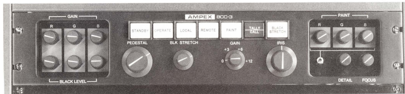
Local Control Unit
